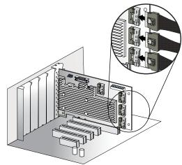
• For adapters with external ports, connect miniSAS HD cables between the adapter and external disk drives or enclosures:
