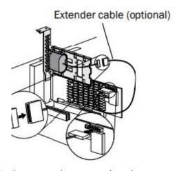
8. Install the mounting plate in the empty slot next to the adapter, as shown in Figure 5-4. After securing the mounting plate to the card cage, verify that the supercapacitor module and mounting plate sit above (and do not touch) the PCIe slot.
