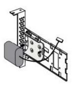
7. Attach the supercapacitor module to the adapter by inserting the connector into the socket on the adapter PCB, as shown in Figure 5-3.
