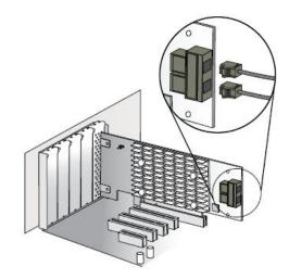
• For a HBA with external ports, connect mini-SAS HD cables between the HBA and external disk drives or enclosures.
