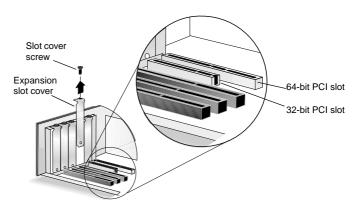
Computers may have vertical or horizontal expansion slots. Refer to your computer manual to locate the PCI/PCI-X slots. If your computer is a tower model, lay it on its side to allow for easier installation of the Adaptec SCSI Card 29320LP.
