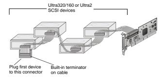
NOTE Internal Ultra320/160 and Ultra2 SCSI devices come from the factory with termination disabled and cannot be changed. Proper termination is provided by the terminator at the end of the LVD SCSI cable.
