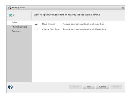
**4.** Select one or more drives. For Move Drives, the wizard displays only physical devices of the same type. For Change Drive Type, the wizard displays only physical devices of a different type. The RAID level determines the number of drives you need to select.
