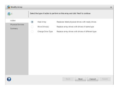
**4.** Select one or more drives to replace the failed drives in the array.
