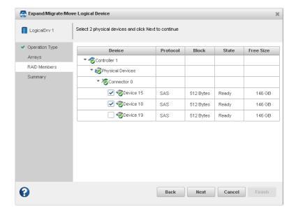
Note: The drives must have sufficient capacity to store the logical drive data.
