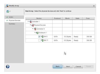
**Note:** The drives must have sufficient capacity to hold all of the logical drives in the array.
