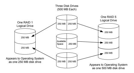
Disk drive space that has been assigned to a logical drive is called a *segment*. A segment can include all or just a portion of a disk drive's space. A disk drive with one segment is part of one logical drive, a disk drive with two segments is part of two logical drives, and so on. When a logical drive is deleted, the segments that comprised it revert to available space (or *free segments*).
