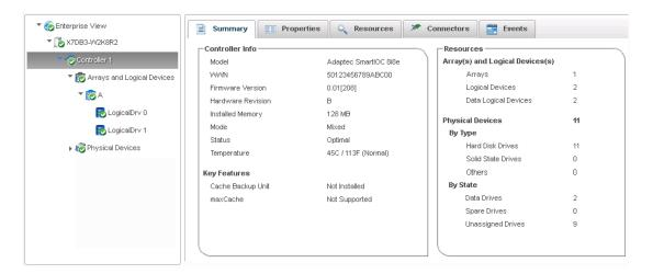
The following table lists the categories and types of information provided on the Storage Dashboard for each component in your storage space. All top-level nodes in the Enterprise View (System, Controller, Arrays, Logical Drives, Physical Devices, and so on) include a Summary tab and Events tab.
