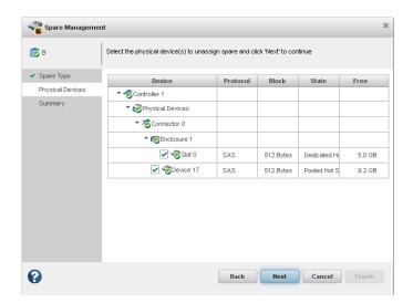
**6.** Review the summary of affected hot spares and arrays, then click **Finish**. If the spare protects only one array, it is deleted and the drive becomes available for other uses in your storage space. If the spare protects more than one array, it is removed from the selected array(s) but continues to protect the other arrays to which it is assigned.
