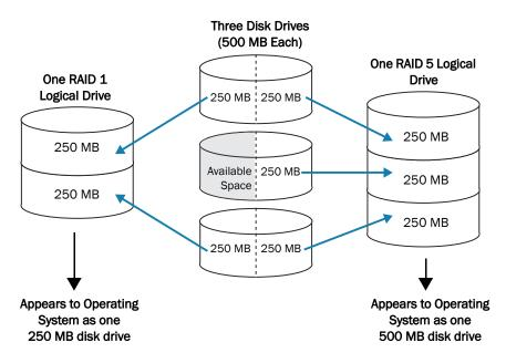
Disk drive space that has been assigned to a logical drive is called a *segment*. A segment can include all or just a portion of a disk drive's space. A disk drive with one segment is part of one logical drive, a disk drive with two segments is part of two logical drives, and so on. A segment can be part of only one logical drive. When a logical drive is deleted, the segments that comprised it revert to available space (or *free segments*).
