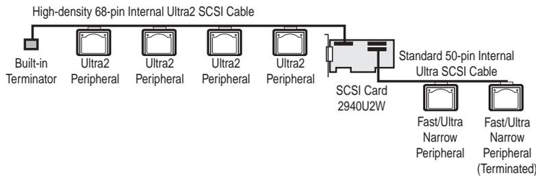
Figure 10. Connecting Ultra2 and Fast/Ultra Narrow Internal Peripherals
