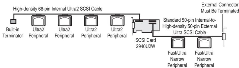
Figure 11. Connecting Ultra2 and Fast/Ultra Narrow Internal Peripherals
