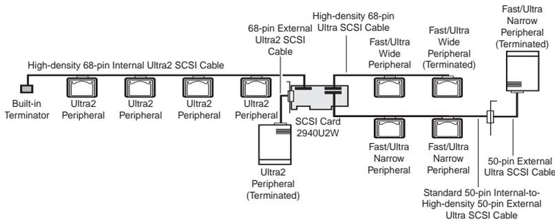
Figure 14. Connecting Ultra2, Fast/Wide Ultra, Fast/Ultra Narrow Internal Peripherals; and Ultra2, Fast/Ultra Narrow External Peripherals
