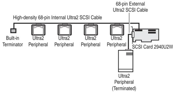
Figure 13. Connecting Ultra2 Internal and External Peripherals
