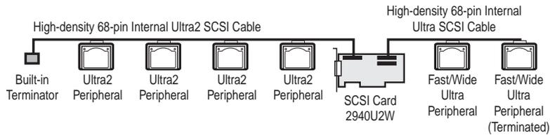
Figure 9. Connecting Ultra2 and Fast/Wide Ultra Internal Peripherals
