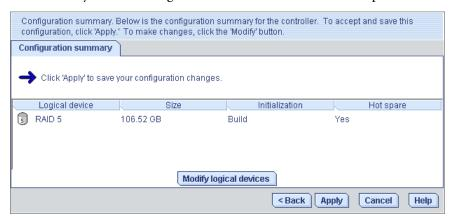
To exclude specific disk drives from the logical drive, specify a size for the logical drive, or to make other changes to the configuration, click Modify logical devices.
