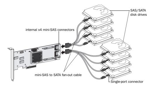
Note: SAS fan-out cables are also available with an additional sideband (SFF-8448) cable that caries SGPIO signals for enclosure management. This additional sideband cable is not used with direct-attached disk drives.
