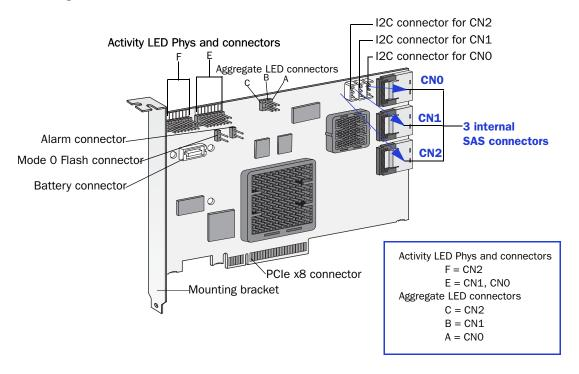
Form Factor Half-size Bus compatibility **PCle** PCIe bus width **8**x PCIe bus speed 2.5 Gb/s
