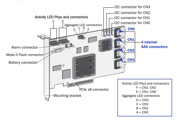
Half-size Form Factor PCle Bus compatibility PCIe bus width х8 PCIe bus speed 2.5 Gb/s Phys (Unified Serial Ports) 16 Standard cache 256 MB DDR2 Connectors, internal 4 mini-SAS x4 (SFF-8087) Maximum number of disk drives 16 (or up to 100 with expanders) I2C and SGPIO **Enclosure Support** Onboard speaker Yes Battery Backup Module Adaptec Battery Module 800 (sold separately—see page 18)
