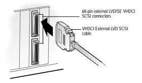
**2** Connect the other end of the cable to a SCSI connector on the back of an external device. If you are installing only one external device, terminate the device and skip to Step 4.
