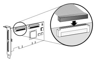
**3** Plug the internal Ultra320/160 and Ultra2 SCSI devices to the other cable connectors, starting with the connector at the terminated end of the cable.
