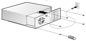
3 Locate an unused 64-bit PCI/PCI-X expansion slot and remove the expansion slot cover. If the computer does not have a 64-bit slot, you can install the card in a 32-bit PCI slot. The Adaptec SCSI Card 39320A supports both 5V and 3.3V 64-bit slots. (The expansion slot must be compliant with PCI Rev. 2.1 or PCI-X Rev. 1.0 and must support Bus Mastering.) Save the slot cover screw for use in Step 4.
