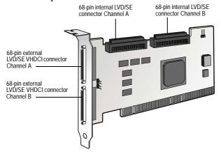
You can connect Ultra320/160 and Ultra2 SCSI devices to the 68-pin LVD connectors on both SCSI channels. When connecting these newer devices along with older *legacy* SCSI devices, Adaptec recommends that you dedicate them as separate channels. See *Support for Older SCSI Devices* on page 2 for more information.
