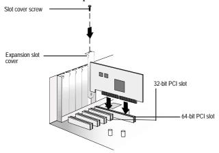
Computers may have vertical or horizontal expansion slots. Refer to your computer manual to locate the PCI/PCI-X slots. If your computer is a tower model, lay it on its side to allow for easier installation of the Adaptec SCSI Card 39320A.
