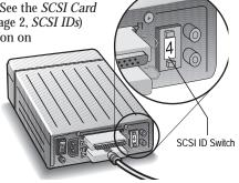
Connect one end of the external SCSI cable to the SCSI Card 1505's external SCSI connector. Secure the cable to the connector on the SCSI Card 1505 by tightening the thumb screws on the cable's connector.
