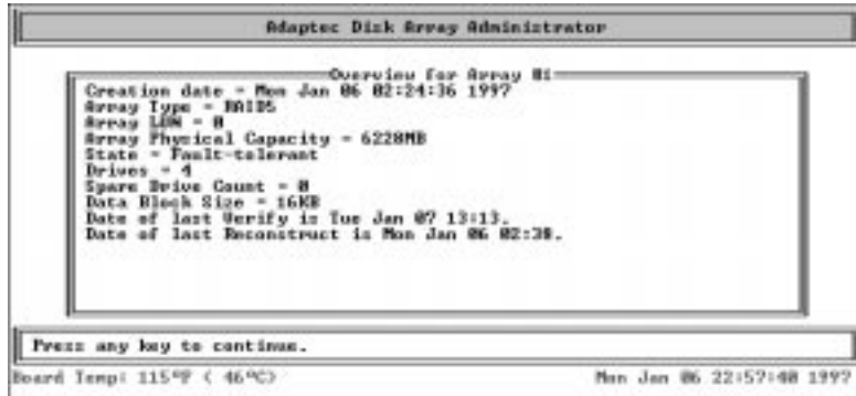
Figure 3-21. Display Array Overview Screen
