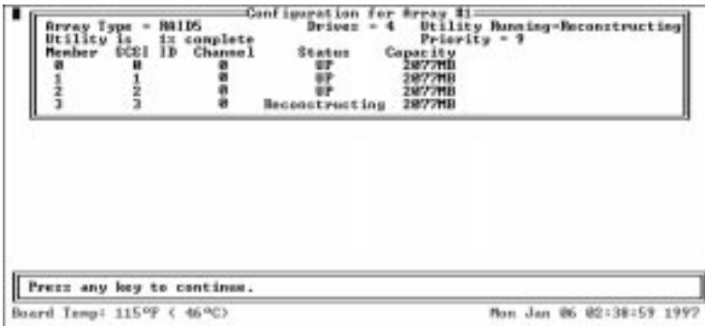
Figure 3-27. Reconstruct In Progress Screen
