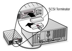
If you are installing only one external device, terminate the device and skip to Step 4.
