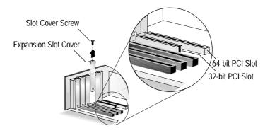
Computers may have vertical or horizontal expansion slots. Refer to your computer manual to locate the PCI slots. If your computer is a tower model, lay it on its side to make it easier to install the Adaptec SCSI Card 29160.
