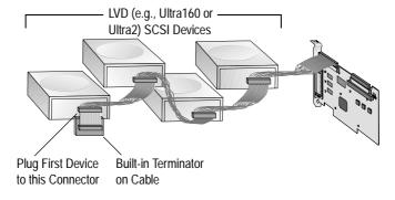
NOTE Internal LVD SCSI devices come from the factory with termination disabled and cannot be changed. Proper SCSI bus termination is provided by the terminator at the end of the LVD SCSI cable. See Terminate the Ends on page 7 for more information.
