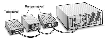
Connect power cables to all external devices and to the computer.
