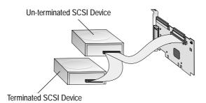
Connect a power cable from your computer's internal power supply to each internal device.
