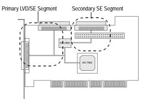
NOTE If you attach Wide Ultra or Ultra SCSI devices to the two connectors on the Primary LVD/SE segment, the data transfer rate for all attached LVD SCSI devices will drop to Ultra SCSI performance levels. However, if you attach *only* LVD SCSI devices to the two connectors on the Primary LVD/SE segment, data will be transferred at the maximum possible rate (80 MBytes/sec for Ultra2 devices and 160 MBytes/sec for Ultra160 devices).
