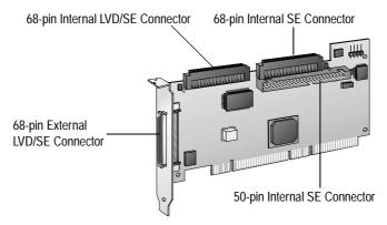
Although the Adaptec SCSI Card 29160 is a 64-bit PCI card, it also works in a 32-bit PCI slot. When installed in a 32-bit PCI slot, the card automatically runs in the slower 32-bit mode.
