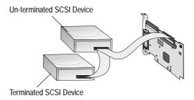
Connect a power cable from your computer's internal power supply to each internal device.
